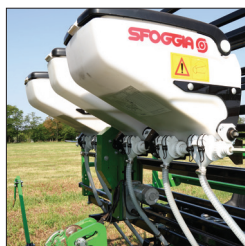
Microgranulator in Pvc, 18 L with 1 exit/volumetric distributor or 32 L with 2 exits/volumetric distributors. Electric transmission or Isobus.
