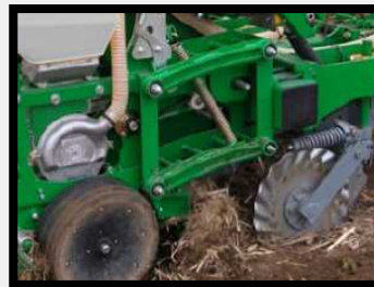
Parallelogram of the planting unit with reinforced arms on bearing (at request). Reinforced row pressing spring
